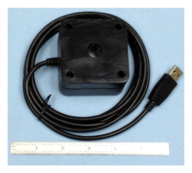
The **USB Interface (USB1312)**, attached to a USB port on a PC running **Sentry Manager** (V10 required), is utilized for **Initialization** of and **Data Recovery** from a **Sentry**.
